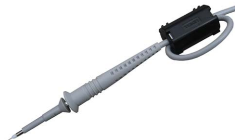
Figure 7-1. Using a ferrite core on the probe cable may help improve probing accuracy
